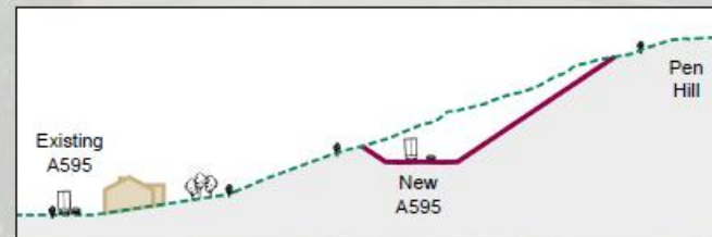
Pen Hill cross-section looking north
