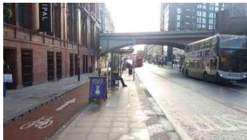
Figure 3.7. Segregated cycleway (carriageway height)
