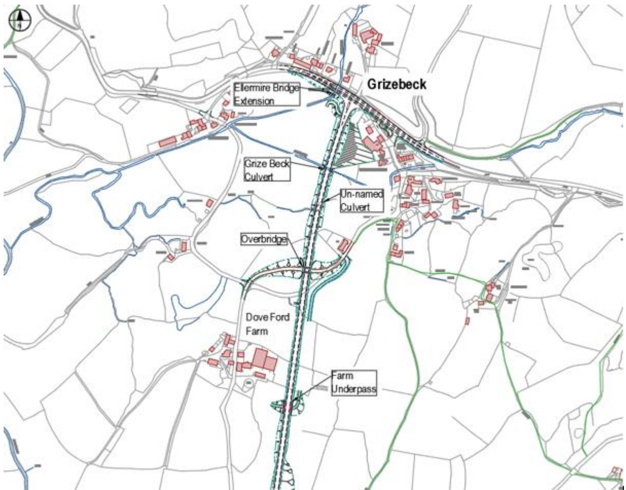
Figure 4: Structural elements included in the scheme
